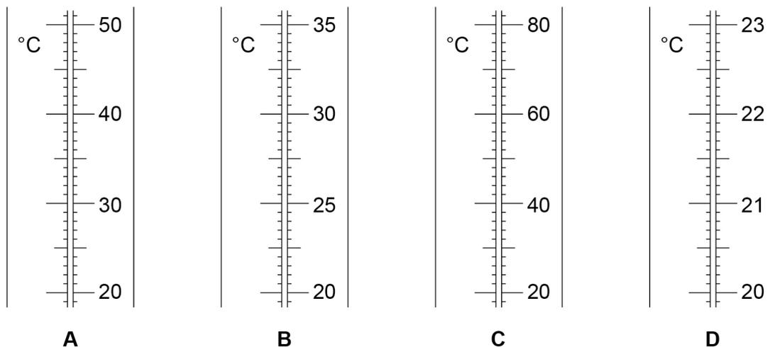
The student wanted to measure the temperature to a resolution of  $0.1\text{ }^{\circ}\text{C}$
